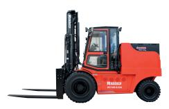
AC80-11 AC120/140-6 AC150/160-6 AC180-6 8,000 kg @ 1,100mm 12,000/14,000 kg @ 600mm 15,000/16,000 kg @ 600mm 18,000 kg @ 600mm
