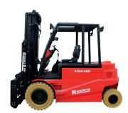
RH 50 5,000 kg @ 600mm RH 60 6,000 kg @ 600mm RH 70 7,000 kg @ 600mm
