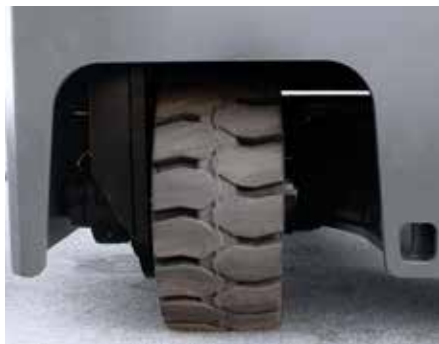
Large diameter wheels in Super Elastic rubber: to operate within industrial buildings and on asphalted floorings. Electromagnetic brakes ensure fast response to the stop command.
